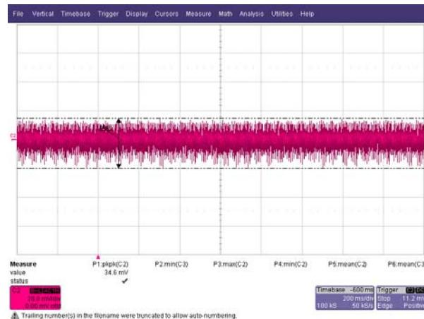
**Figure 27** – Ripple [35 mV<sub>PP</sub>], 115 VAC, Full Load.
