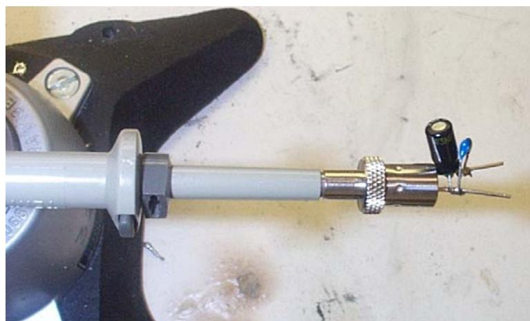
**Figure 25** – Oscilloscope Probe with Probe Master ([www.probmast.com](http://www.probmast.com)) 4987A BNC Adapter.
