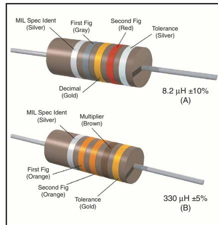
**Fig 24.4—Color coding for tubular encapsulated RF chokes. At A, an example of the coding for an 8.2- $\mu$ H choke is given. At B, the color bands for a 330- $\mu$ H inductor are illustrated. The color code is given in [Table 24.2](#).**
