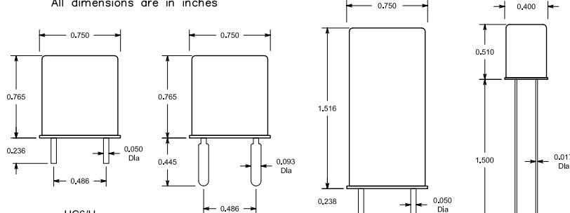
\* Note: HC17/U pin spacing and diameter is equivalent to the older FT-243 (32 pF) holder.
