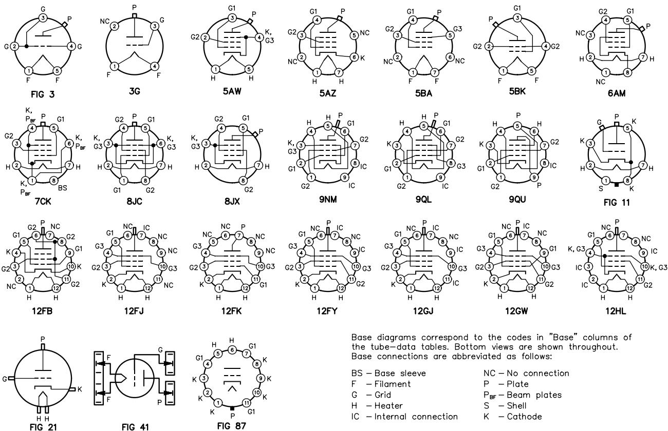
Base diagrams correspond to the codes in "Base" columns of the tube-data tables. Bottom views are shown throughout. Base connections are abbreviated as follows:
