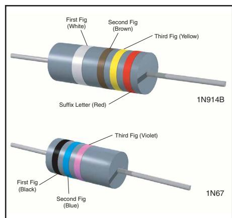
**Fig 24.5—Color coding for semiconductor diodes. At A, the cathode is identified by the double-width first band. At B, the bands are grouped toward the cathode. Two-figure designations are signified by a black first band. The color code is given in Table 24.2. The suffix-letter code is A—Brown, B—red, C—orange, D—yellow, E—green, F—blue. The 1N prefix is understood.**
