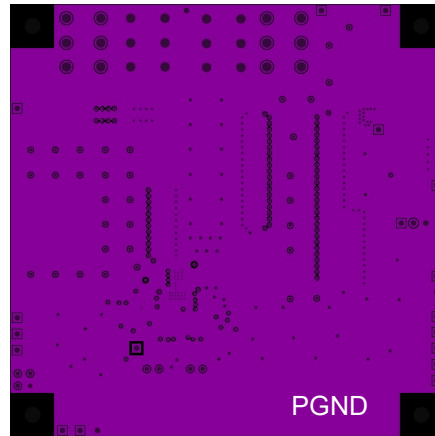
Figure 51c: IRDC3846 Demo board Layout Considerations – Mid Layer 1
