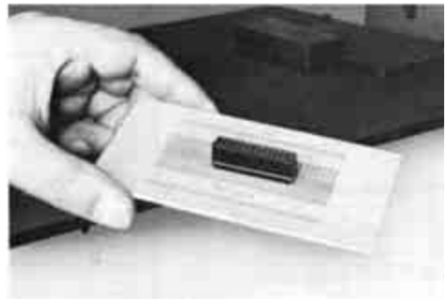
6. Now connector has been mounted to the board securely.
