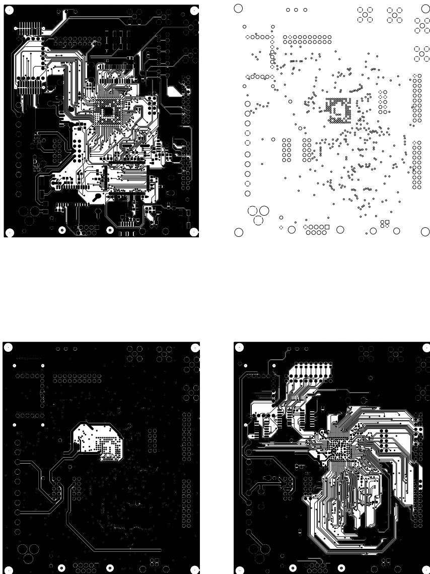
**Figure 10: CC2400EB PCB layout, layer 1 (top left), layer 2 (top right), layer 3 (bottom left) and layer 4 (bottom right)**
