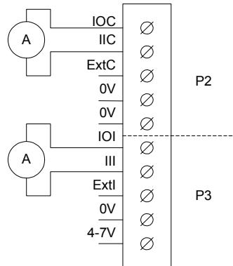
**Figure 8: Power terminal block with amperemeters attached**
