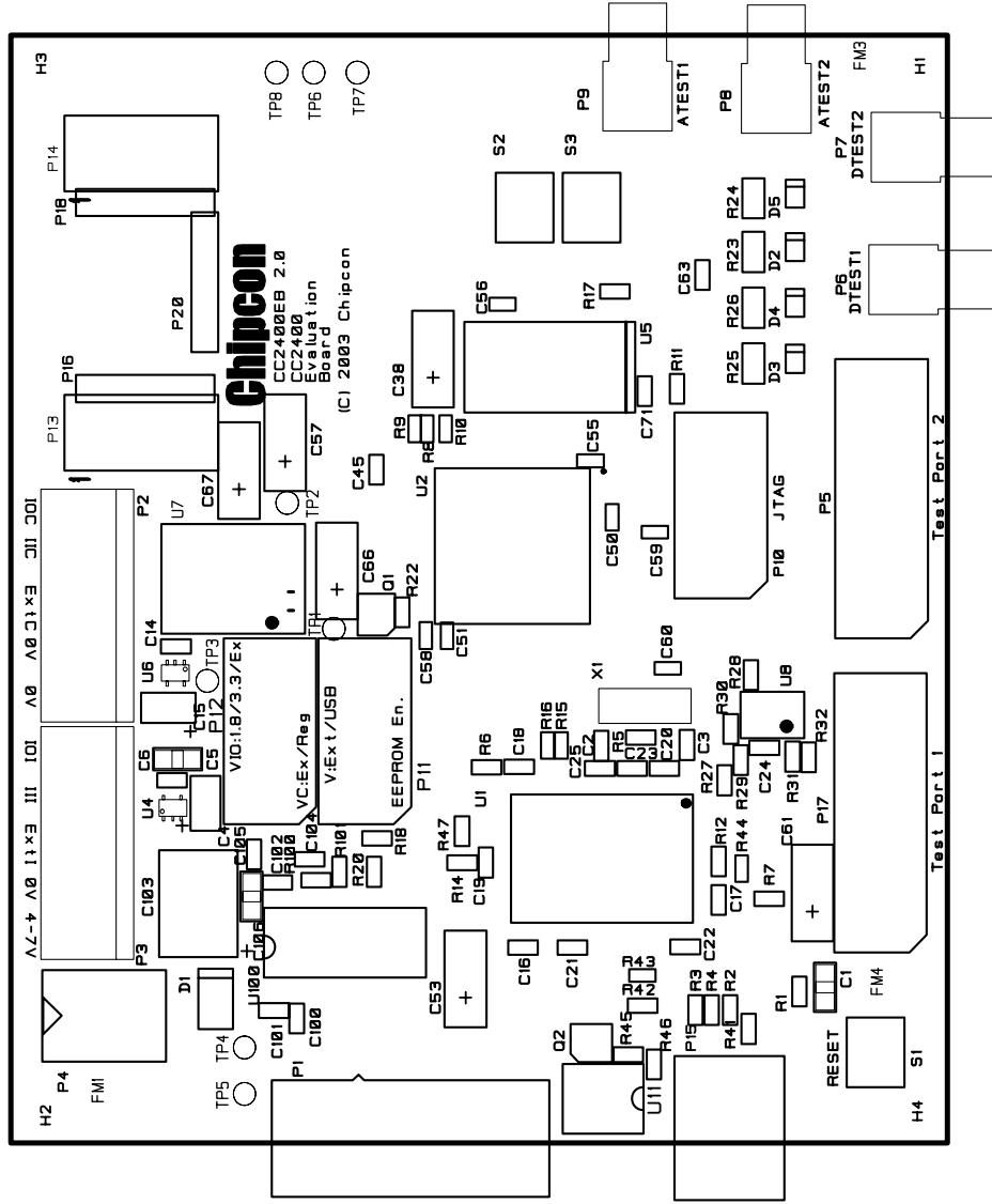
**Figure 11: CC2400EB component placement, top side**
