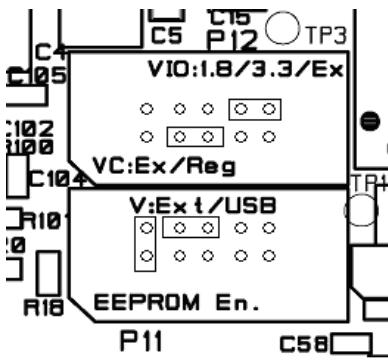
Figure 9b CC2420 internal voltage regulator selected on CC2420EM
