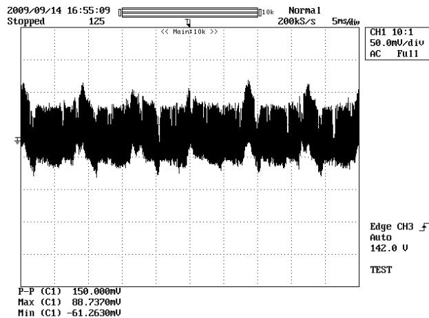
**Figure 34 – Ripple, 115 VAC, Full Load.**
