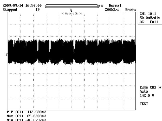
**Figure 36 – Ripple, 265 VAC, Full Load.**
