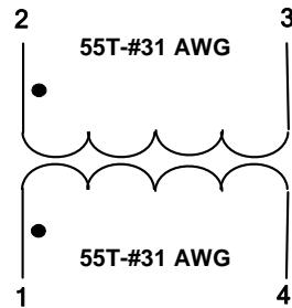
**Figure 8 – CMC Electrical Diagram.**
