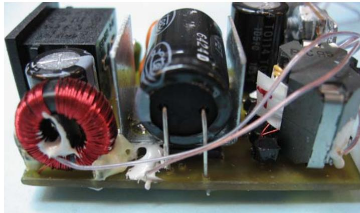
**Figure 19** – Thermocouple on CMC and IC SOURCE Pin.
