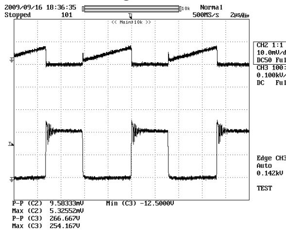
**Figure 22 – 85 VAC, 50Hz Full Load.**
