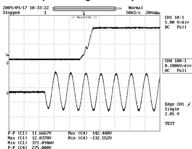
**Figure 24 – Start-up Profile, 90 VAC, 50 Hz**
