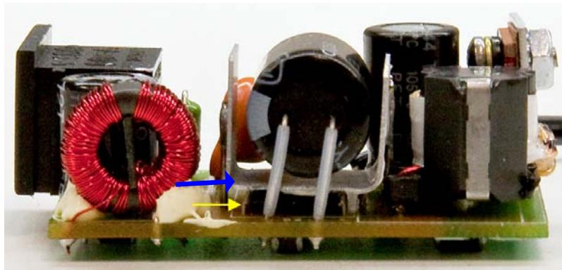
Figure 2 – Side View Showing TOP264VG V-Package with Heatsink Mounted on Top.
