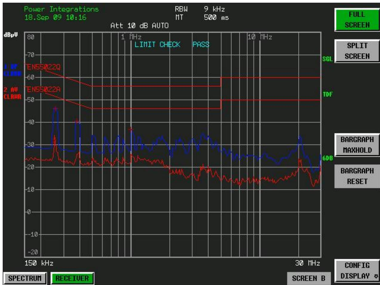
**Figure 45** – Conducted EMI, Maximum Steady State Load, 230 VAC, 60 Hz, and EN55022 B Limits.
