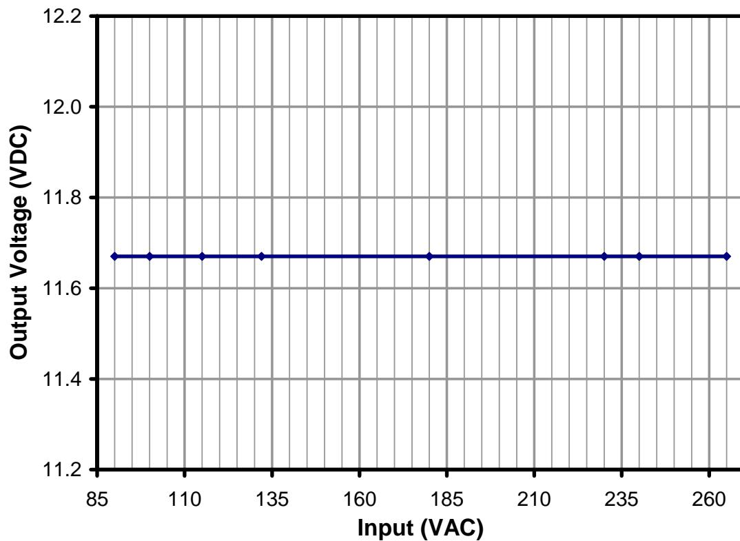
**Figure 17 – Line Regulation, Room Temperature, Full Load.**
