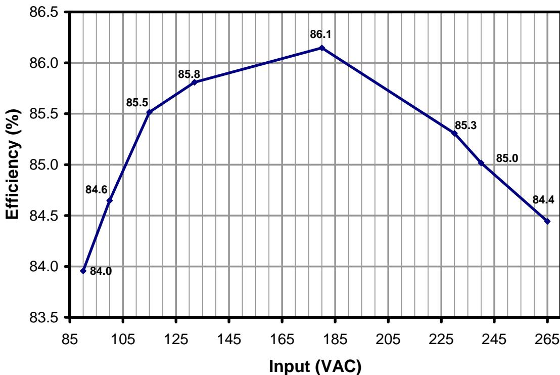
**Figure 12 – Efficiency vs. Input Voltage, Room Temperature, 60 Hz.**
