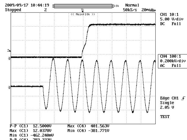
**Figure 25 – Start-up Profile, 265 VAC, 50 Hz**
