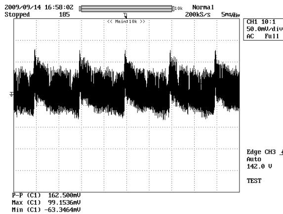
**Figure 33 – Ripple, 90 VAC, Full Load.**
