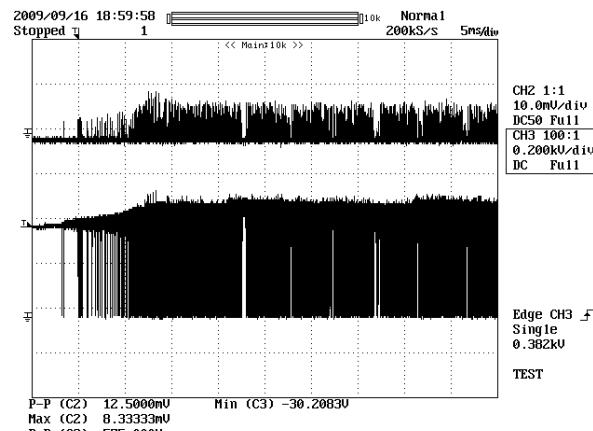
**Figure 27 – 265 VAC Input and Maximum Load.**
