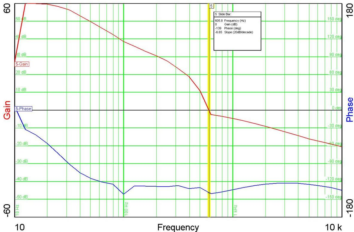
**Figure 42** – Gain-Phase Plot, 265 VAC, Maximum Steady State Load.
