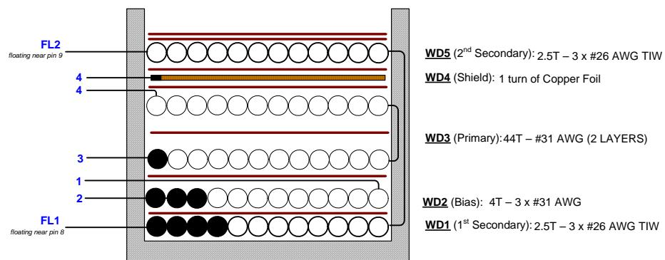
Figure 6 – Transformer Build Diagram.
