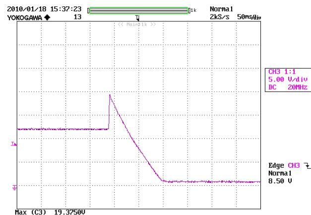
**Figure 38 – 230 VAC; 12 V Output 100 mA Load.**
