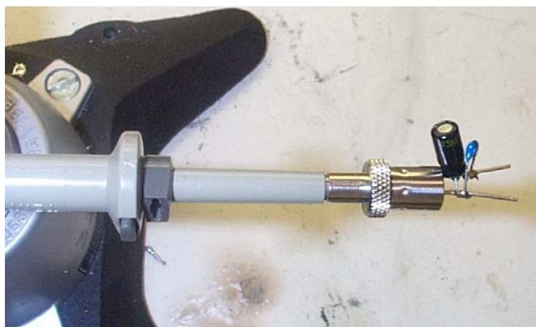
Figure 32 – Oscilloscope Probe with Probe Master ([www.probemaster.com](http://www.probemaster.com)) 4987A BNC Adapter.
