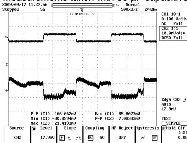
**Figure 29 – Transient Response, 90 VAC, 50 Hz**
