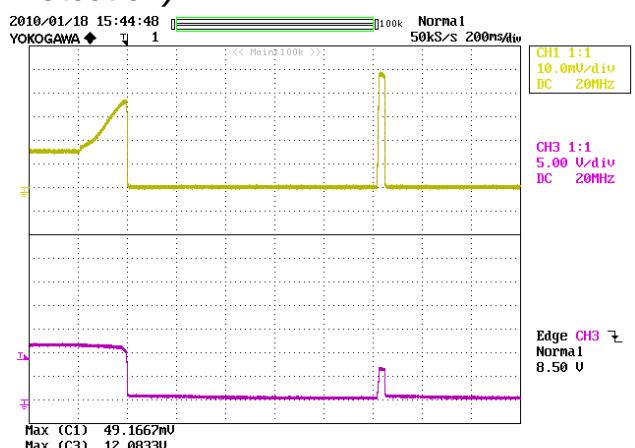
**Figure 40 – 265 VAC Input and Maximum Load.**
