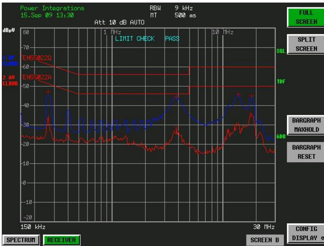
**Figure 44** – Conducted EMI, Maximum Steady State Load, 115 VAC, 60 Hz, and EN55022 B Limits.
