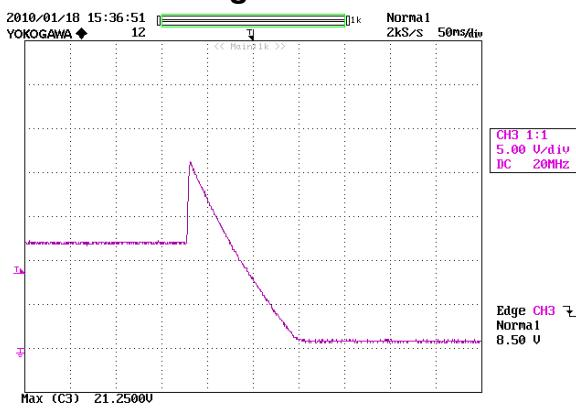
**Figure 37 – 115 VAC; 12 V Output 100 mA Load.**
