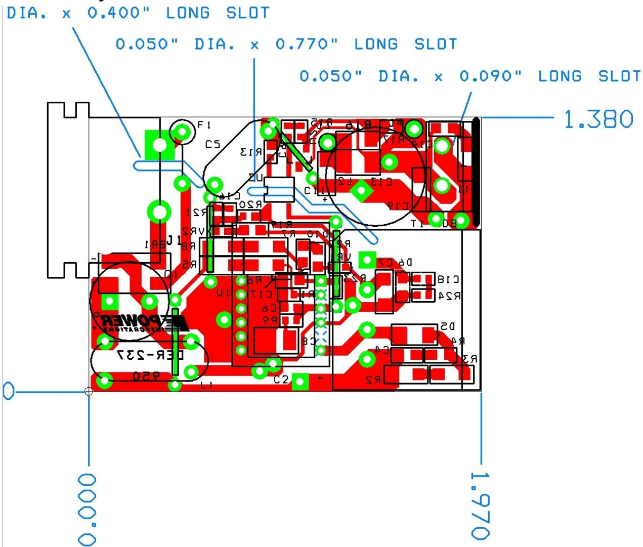
Figure 4 – Printed Circuit Layout (35 mm x 50 mm).
