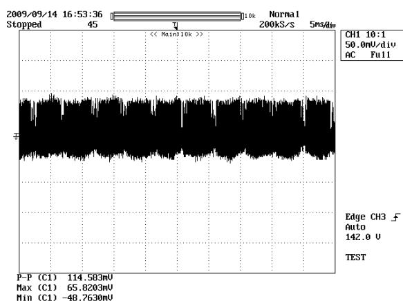
**Figure 35 – Ripple, 230 VAC, Full Load.**
