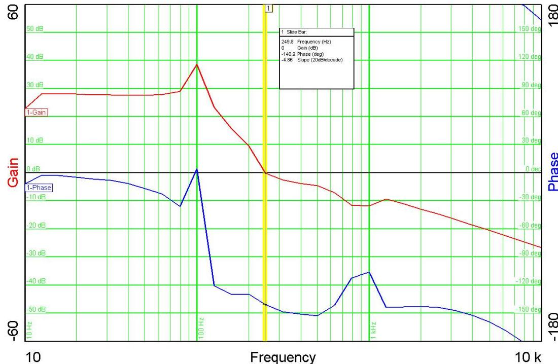
**Figure 41 – Gain-Phase Plot, 90 VAC, Maximum Steady State Load.**
