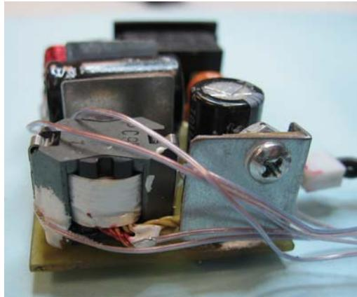
**Figure 20** – Thermocouple on Transformer Core, Transformer Winding, Output Diode.
