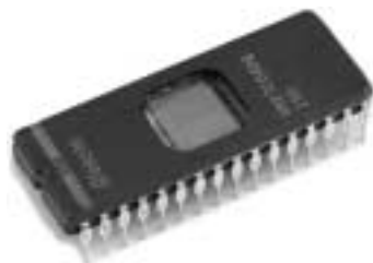
Ceramic Dual-in-Line Package (CerDIP) Product Suffix: J
