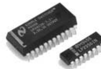
Molded Dual-in-Line Package (DIP) Product Suffix: N
