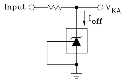
Example :  $\Delta V_{ref} = 8.0\text{mV}$  and slope is positive,  $V_{ref}$  at  $25^\circ\text{C} = 2.495\text{V}$ ,  $\Delta T_a = 70^\circ\text{C}$
