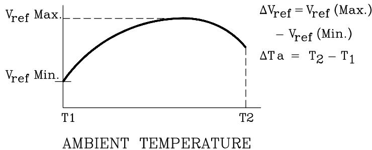
The average temperature coefficient of the Reference input voltage,  $\alpha V_{ref}$ , is defined as:
