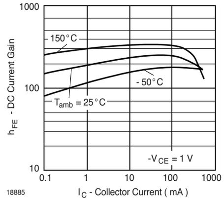
Fig. 5 DC Current Gain vs. Collector Current
