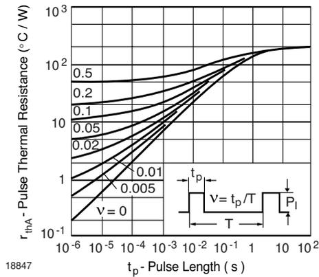
Fig. 2 Pulse Thermal Resistance vs. Pulse Duration
