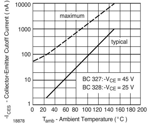
Fig. 4 Collector-Emitter Cutoff Current vs. Ambient Temperature
