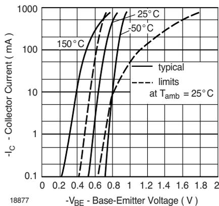
Fig. 3 Collector Current vs. Base-Emitter Voltage
