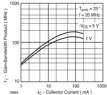
Fig. 11 Gain-Bandwidth Product vs. Collector Current
