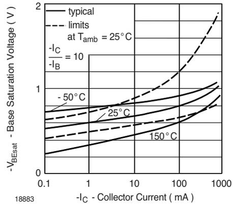
Fig. 10 Base Saturation Voltage vs. Collector Current
