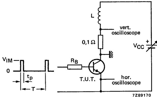
Fig. 4 Test circuit for turn-off breakdown energy.
