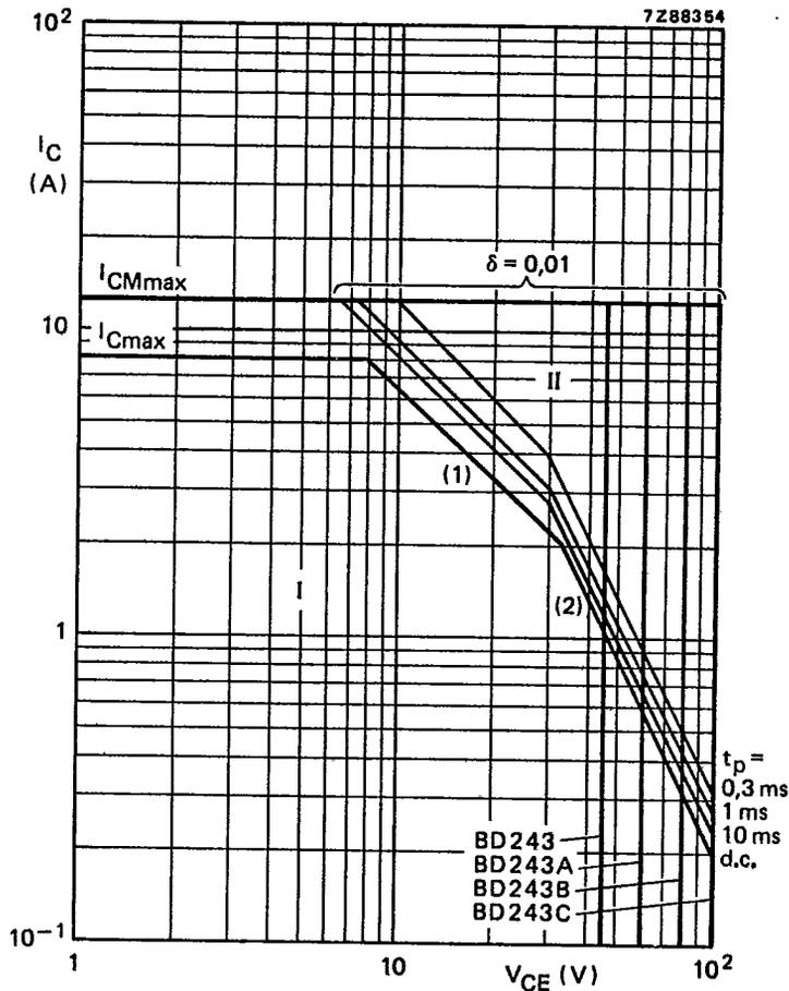
Fig. 5 Safe Operating Area;  $T_{mb} = 25\text{ }^{\circ}\text{C}$ .
