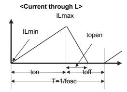
Step 1: Lx Tr. turns on and current IL (=i1) flows, and energy is charged into CL. At this moment, IL increases from ILmin. (=0) to reach ILmax. in proportion to the on-time period(ton) of LX Tr.
