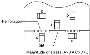
1-3. When PCB is split, the amount of mechanical stress on the capacitors can vary according to the method used. The following methods are listed in order from least stressful to most stressful: push-back, slit, V-grooving, and perforation. Thus, please consider the PCB, split methods as well as chip location.
