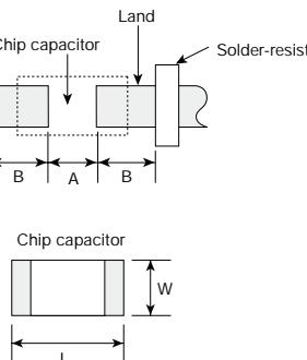
Array type: Recommended land dimensions for reflow-soldering ( unit: mm )
