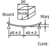
Capacitance measurement shall be conducted with the board bent
