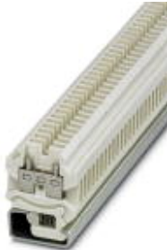
Feed-through terminal block, connection method: screw connection, cross section: 0.2 mm 2 - 4 mm 2 , 24 - 12 AWG, width: 6.2 mm, color: white, mounting type: NS 32, insulation material: ceramic
