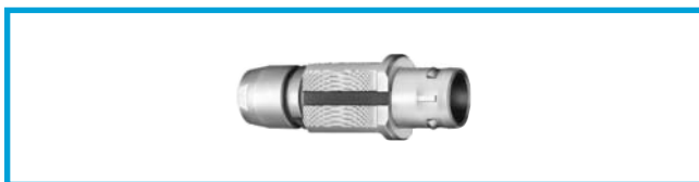
FIG Straight plug for remote handling, key (G) or keys (A...L and R), special alignment mark, knurled handling surface, cable collet
