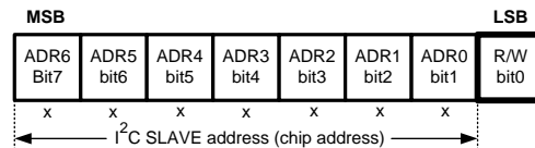
Figure 16. I 2 C Chip Address (0x2C)
