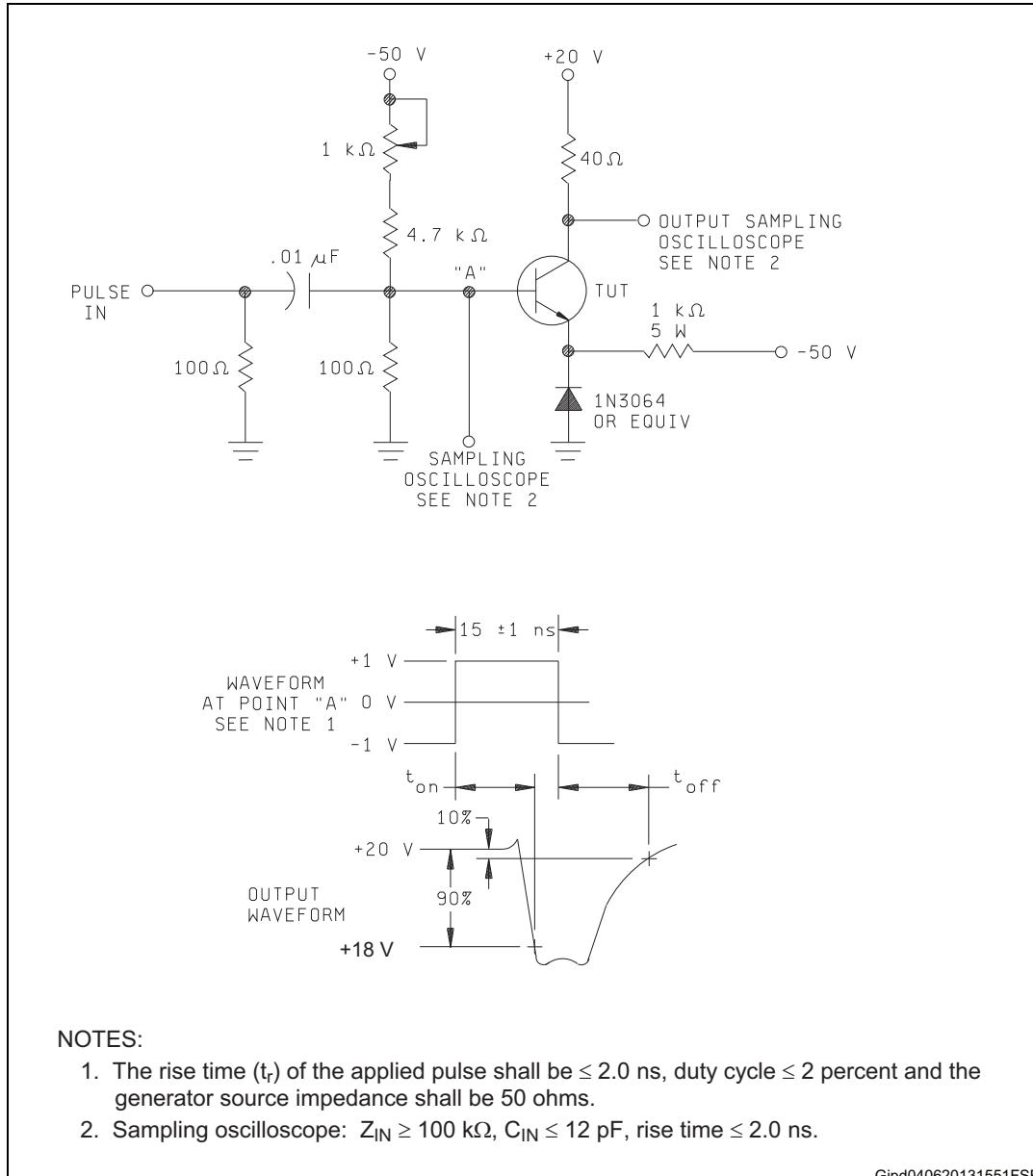
**Figure 7. ESCC resistive load switching test circuit**
