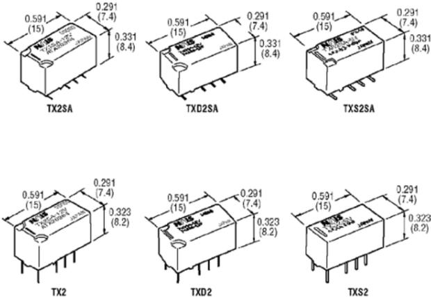
2 amp. Breakdown Voltage: 2000 V between contacts and coil. Surge Voltage Withstand: 2500 V (Bellcore). 2 Form C contact arrangement. TXD is high insulation type; TXS is high sensitivity type. Operating Temperature: -40°C to +85°C. UL/CSA.
