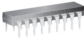
18-pin DIP (A package)
