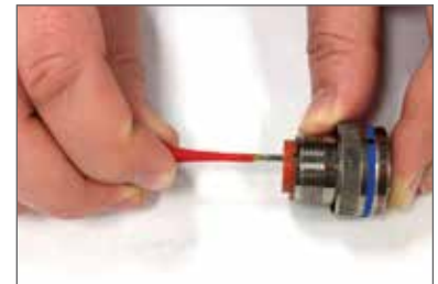
Plastic tool with contact in proper position.
