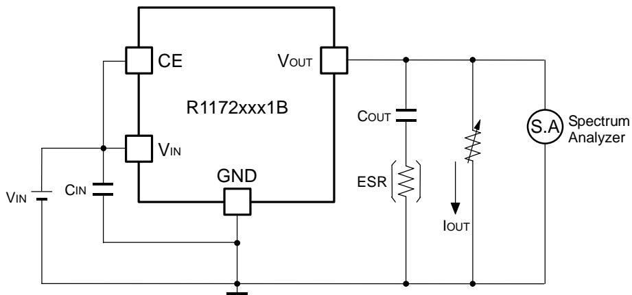
0.8V to 3.3V Output type:  $C_{OUT}=4.7\mu F$  (Kyocera CM105X5R475M06AB)
