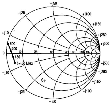
**Figure 16.  $S_{11}$ , Input Reflection Coefficient
