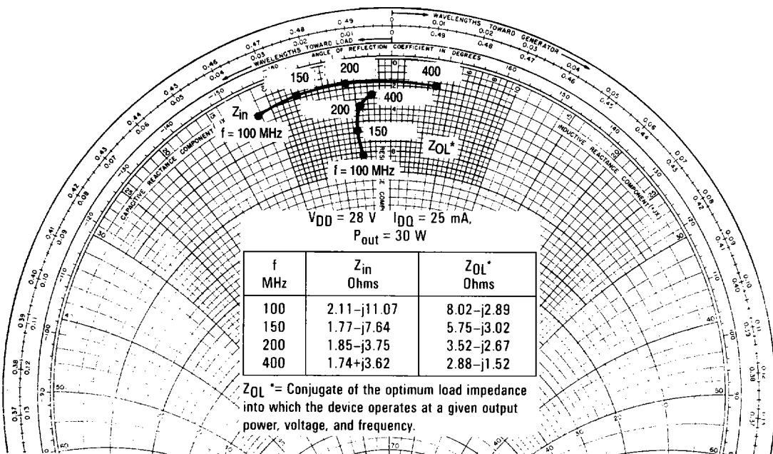
Figure 15. Large-Signal Series Equivalent Input and Output Impedance, Z<sub>in</sub>, Z<sub>OL\*</sub>
