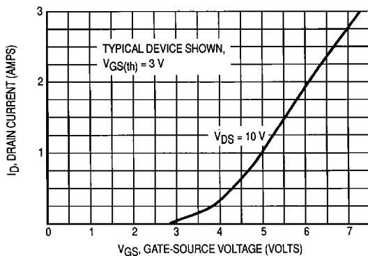
**Figure 10. Drain Current versus Gate Voltage (Transfer Characteristics)**
