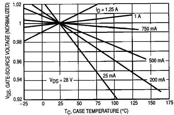
**Figure 11. Gate Source Voltage versus Case Temperature**
