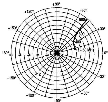
**Figure 17.  $S_{12}$ , Reverse Transmission Coefficient
