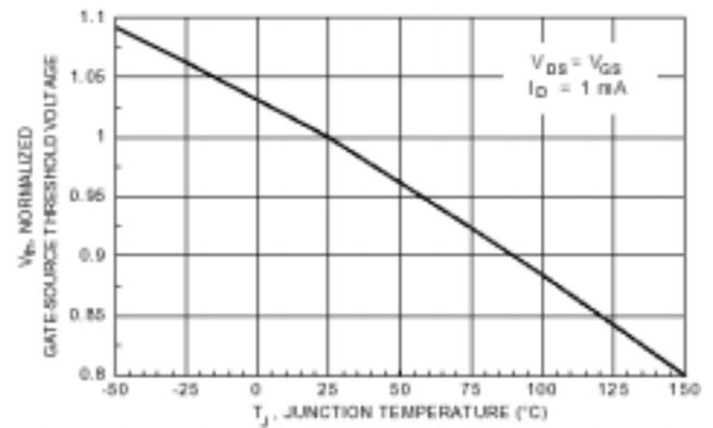
Figure 6. Gate Threshold Variation with Temperature.
