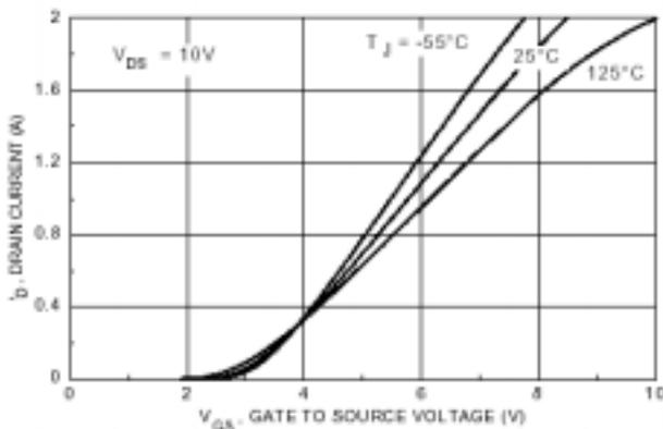
Figure 5. Transfer Characteristics.
