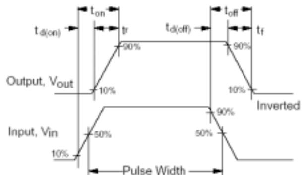
Figure 12. Switching Waveforms.
