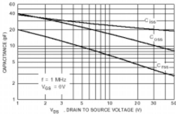
Figure 9. Capacitance Characteristics
