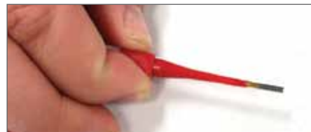
Plastic tool with contact in proper position.
