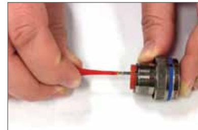
Plastic tool with contact in proper position.
