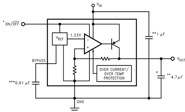
\*ON/OFF input must be actively terminated. Tie to  $V_{IN}$  if this function is not to be used.
