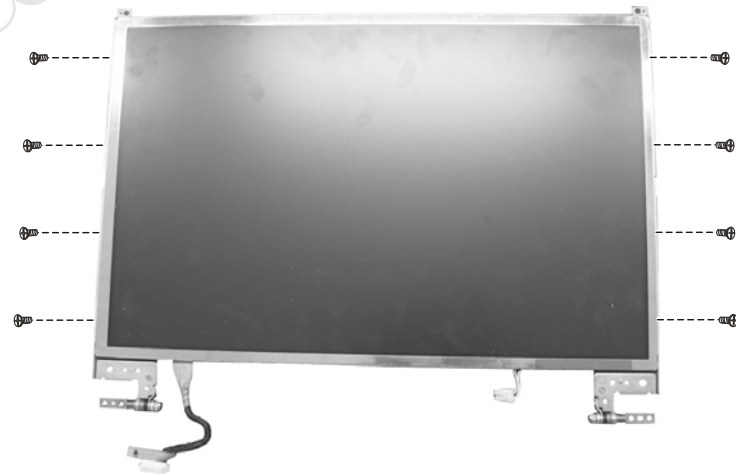
Figure 2-19 Remove eight screws
