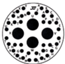
25-42 - 25-42* 38 #20, 4 #8 Coax I, Coax
