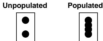
**Figure 4. Two-Terminal Jumper**
