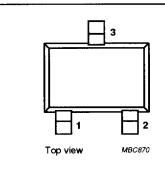
Fig.1 Simplified outline (SOT323) and pin configuration.
