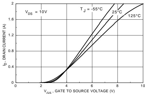
**Figure 5. Transfer Characteristics**
