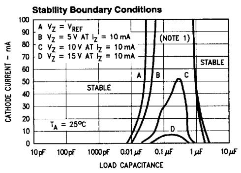
Note 1: The areas under the curves represent conditions that may cause the device to oscillate. For curves B, C, and D, R2 and  $V^+$  were adjusted to establish the initial  $V_Z$  and  $I_Z$  conditions with  $C_L = 0\text{ V}^+$  and  $C_L$  were then adjusted to determine the ranges of stability.
