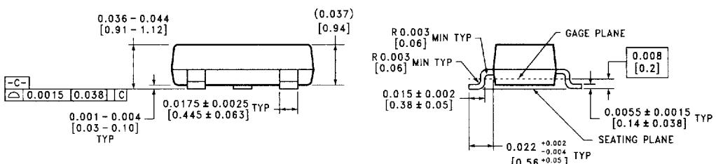
SOT-23 Molded Small Outline Transistor Package (M3)
