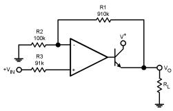
$V_0 = 0 \ V_{DC}$  for  $V_{IN} = 0 \ V_{DC}, \, A_V = 10$
