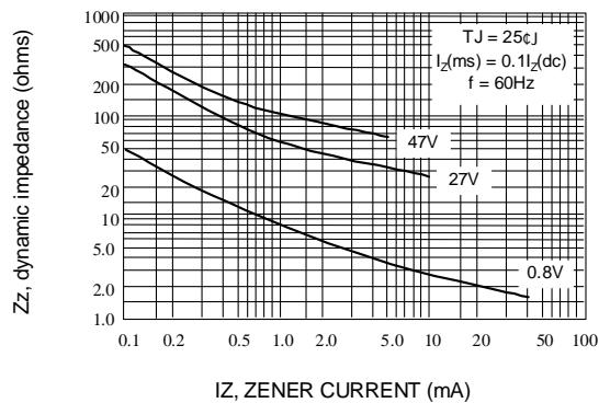
Fig. 6-EFFECT OF ZENER CURRENT ON ZENER IMPEDANCE
