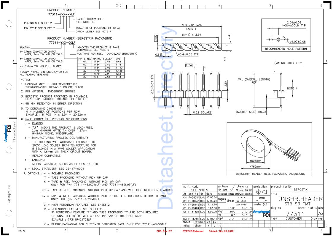
213 PLATING 1 = 0.76µm GOLD/GXT ON CONTACT AREA, 2µm TIN MIN ON TAIL  $4 = 2\mu m$  TIN MIN FULL PLATED 5 = 0.25µm GOLD/GXT ON CONTACT AREA, 2µm TIN MIN ON TAIL
