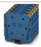
High-current terminal block, with test socket, nom. voltage: 1000 V AC / 1500 V DC, nominal current: 232 A, connection method: Power-Turn connection, number of connections: 2, number of positions: 1, cross section: 25 mm² - 95 mm², AWG: 4 - 4/0, width: 25 mm, color: blue, mounting type: NS 35/15
