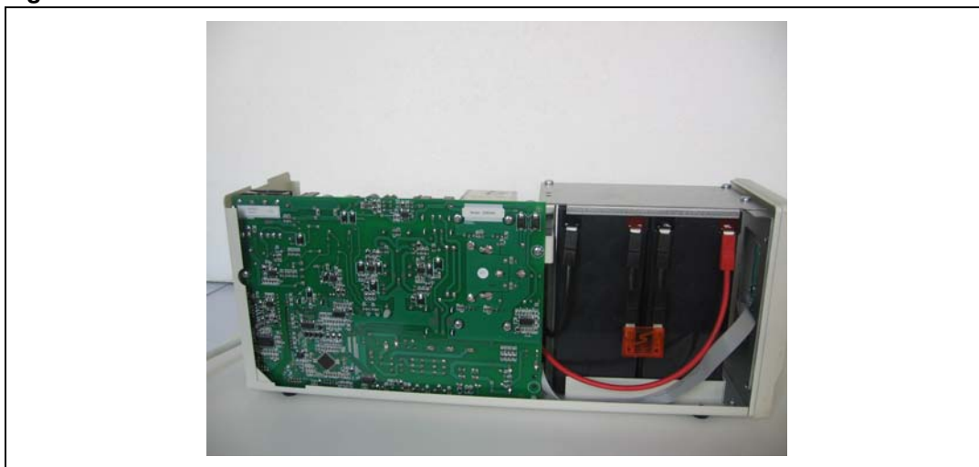
Figure 35. UPS fully assembled
