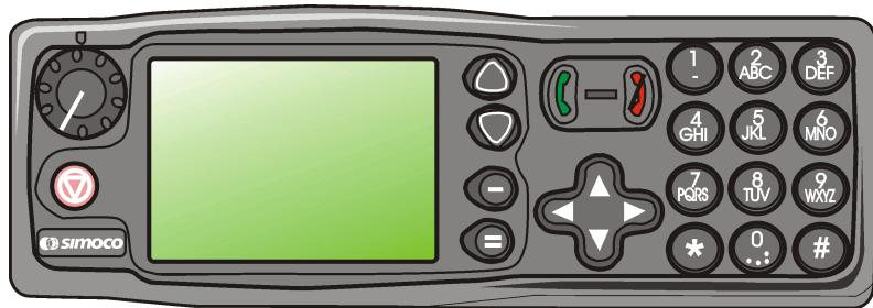
Figure E.1 SRM9030 Control Head
