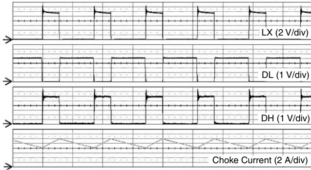
2 \mu s/div V_{IN} = 12 V, V_{OUT} = 3.3 V, Load Current = 10 A, L = 2.2 \mu H, C_{OUT} = 100 \mu F x 3 Typical Switching Waveform
