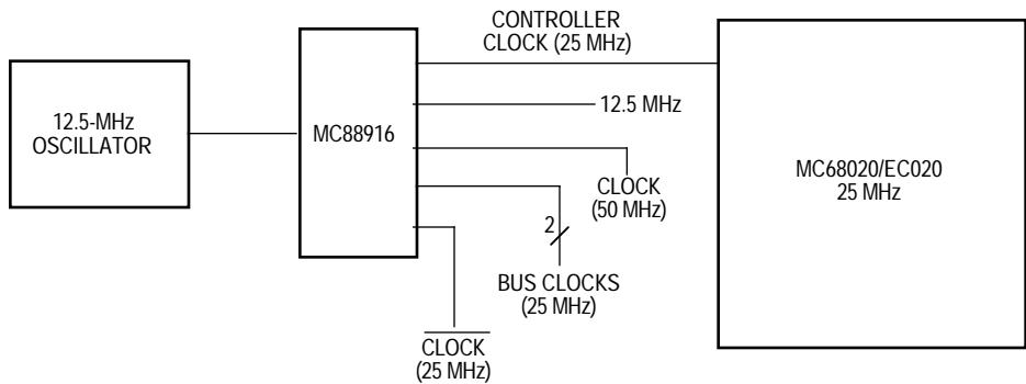
**Figure 9-7. High-Resolution Clock Controller**
