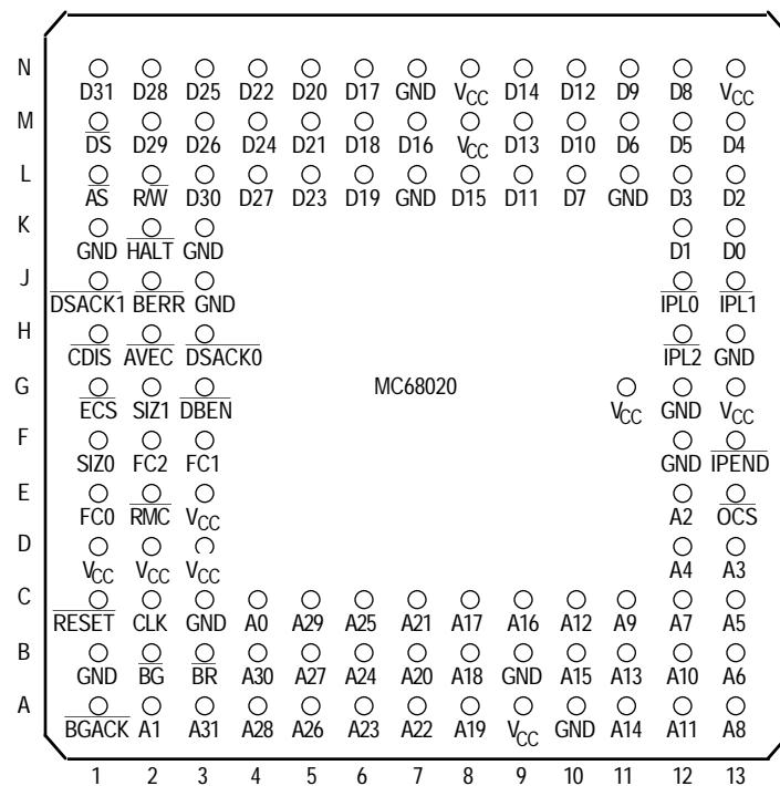
The V<sub>CC</sub> and GND pins are separated into four groups to provide individual power supply connections for the address bus buffers, data bus buffers, and all other output buffers and internal logic. It is recommended that all pins be connected to power and ground as indicated.
