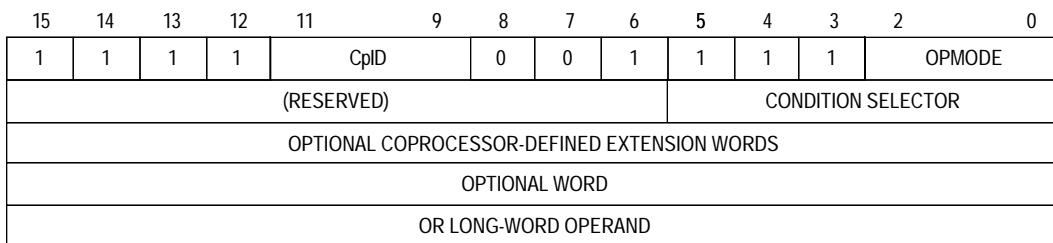
**Figure 7-13. Trap on Coprocessor Condition Instruction Format (cpTRAPcc)**
