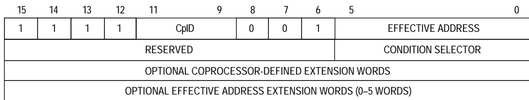
**Figure 7-11. Set on Coprocessor Condition Instruction Format (cpScc)**
