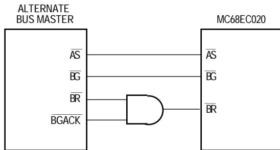
**Figure 5-50. Interface for Three-Wire to Two-Wire Bus Arbitration**
