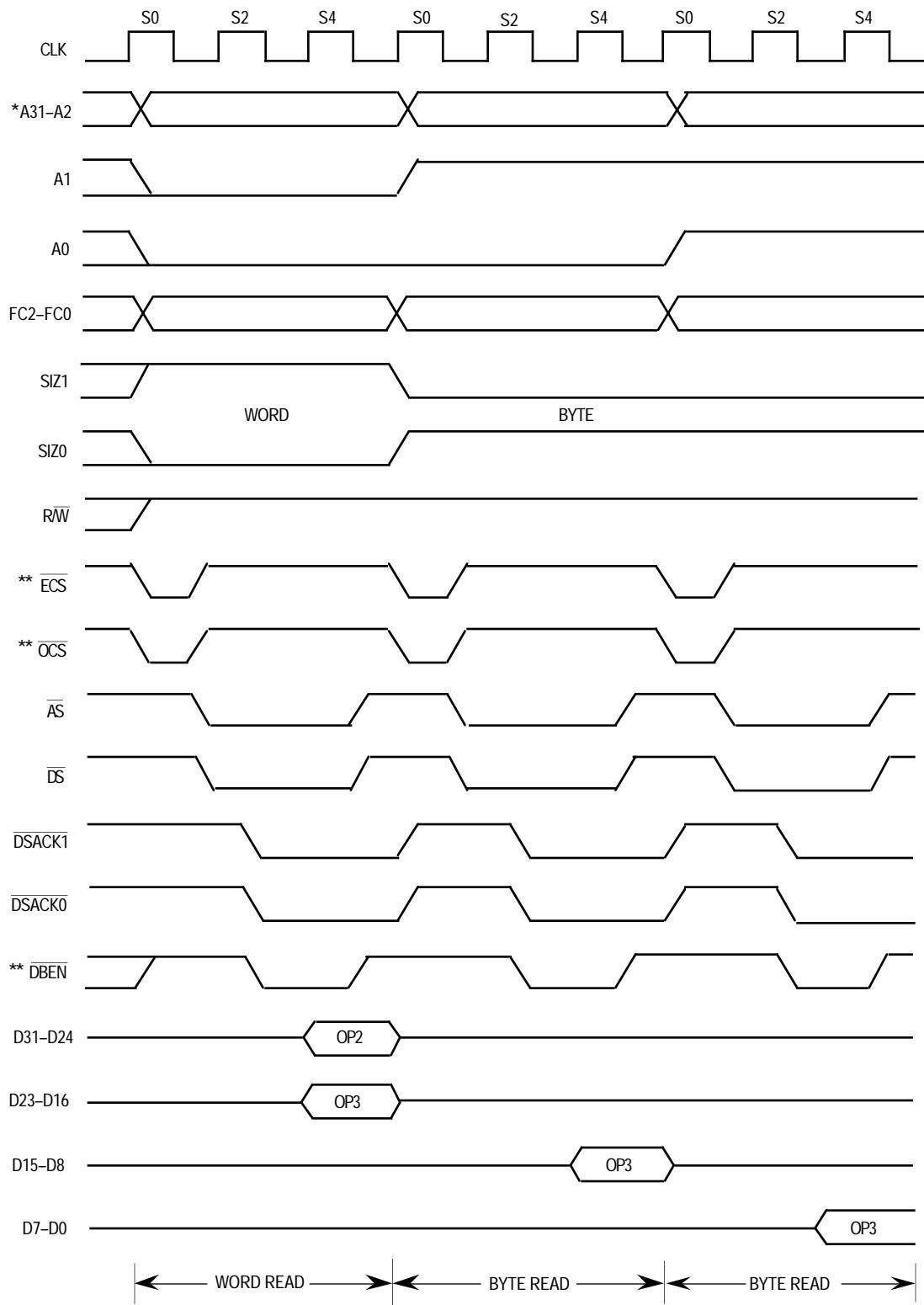
**Figure 5-21. Byte and Word Read Cycles—32-Bit Port**
