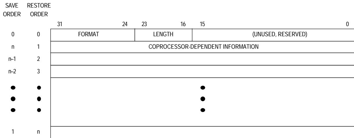
**Figure 7-14. Coprocessor State Frame Format in Memory**
