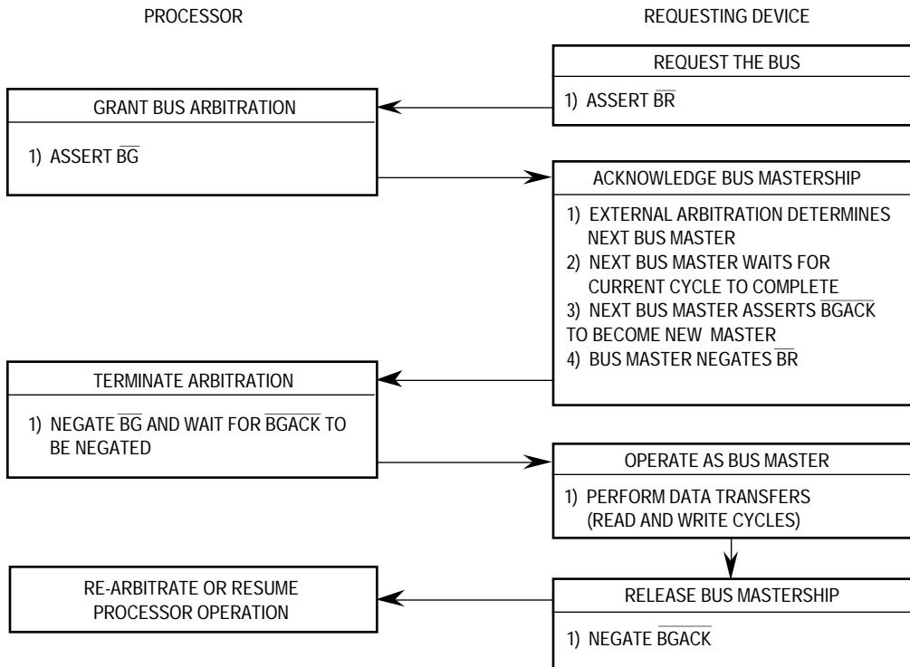
**Figure 5-42. MC68020 Bus Arbitration Flowchart for Single Request**
