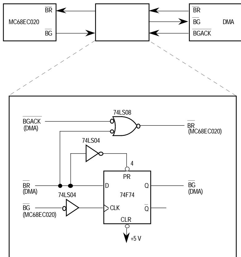
**Figure A-1. Bus Arbitration Circuit—
