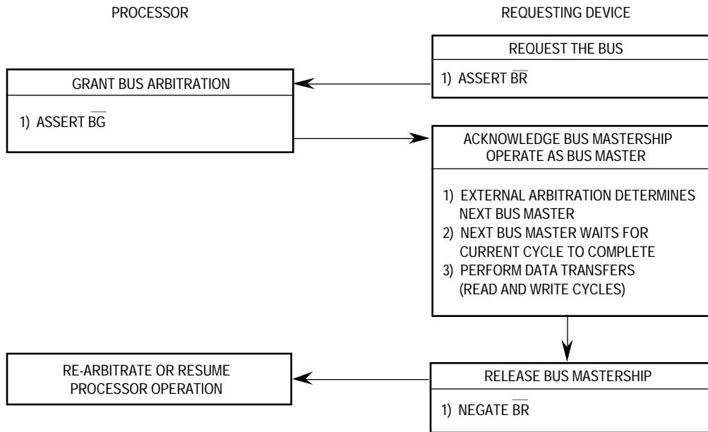
**Figure 5-46. MC68EC020 Bus Arbitration Flowchart for Single Request**
