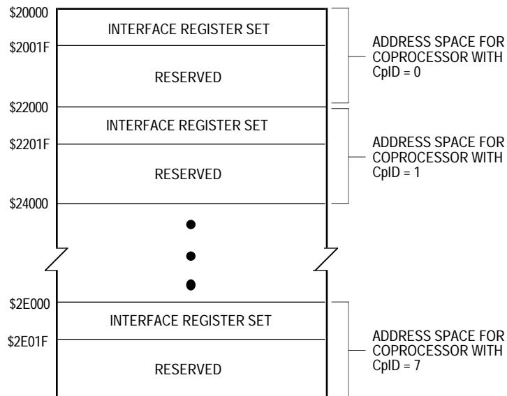
**Figure 7-4. Coprocessor Address Map in MC68020/EC020 CPU Space**
