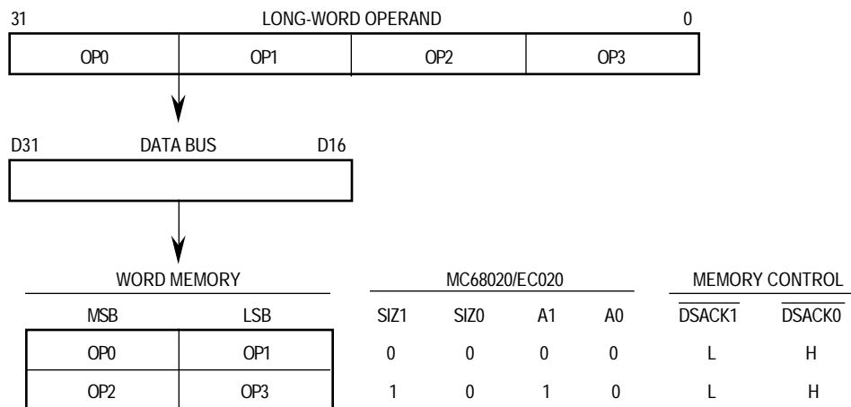
**Figure 5-5. Long-Word Operand Write to Word Port Example**
