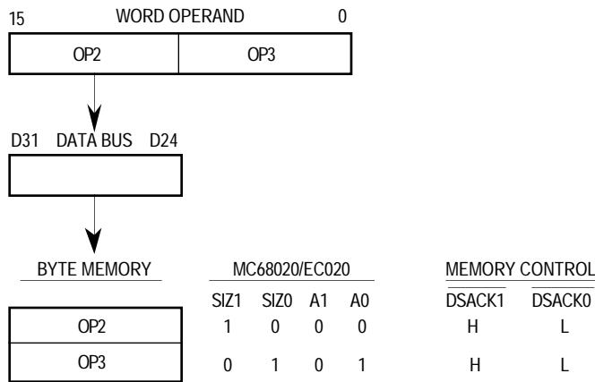
**Figure 5-7. Word Operand Write to Byte Port Example**
