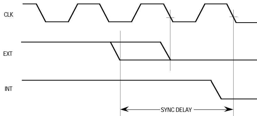
**Figure 5-1. Relationship between External and Internal Signals**
