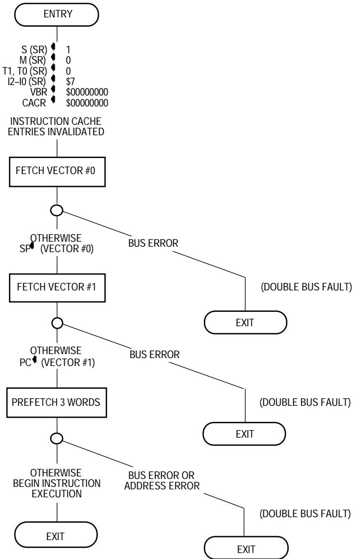
**Figure 6-1. Reset Operation Flowchart**
