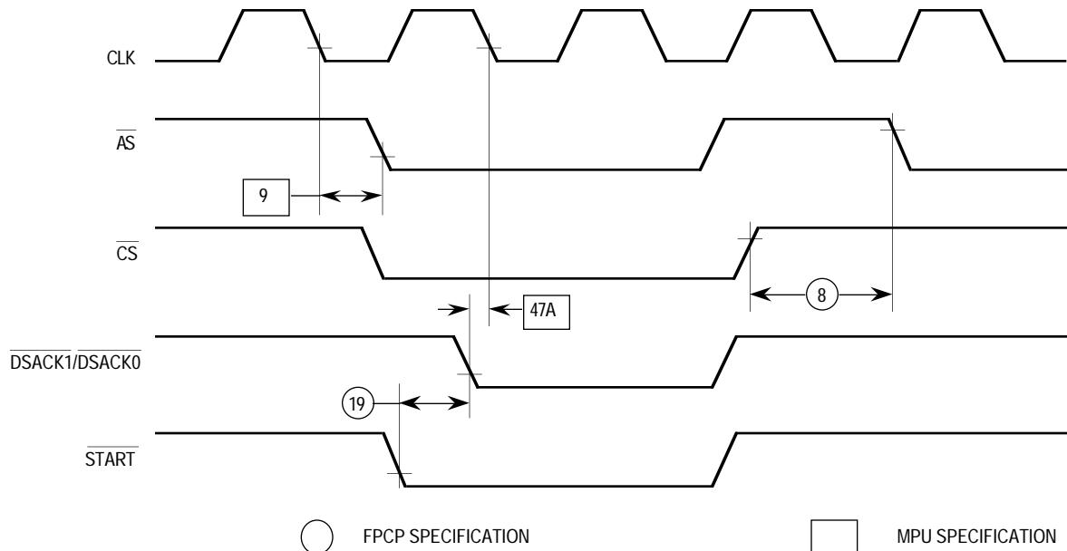
**Figure 9-4. Bus Cycle Timing Diagram**
