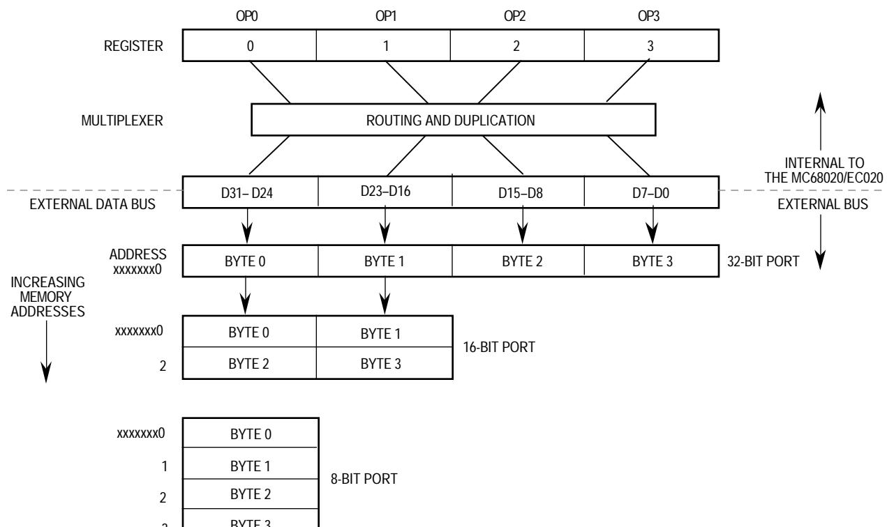
**Figure 5-4. MC68020/EC020 Interface to Various Port Sizes**
