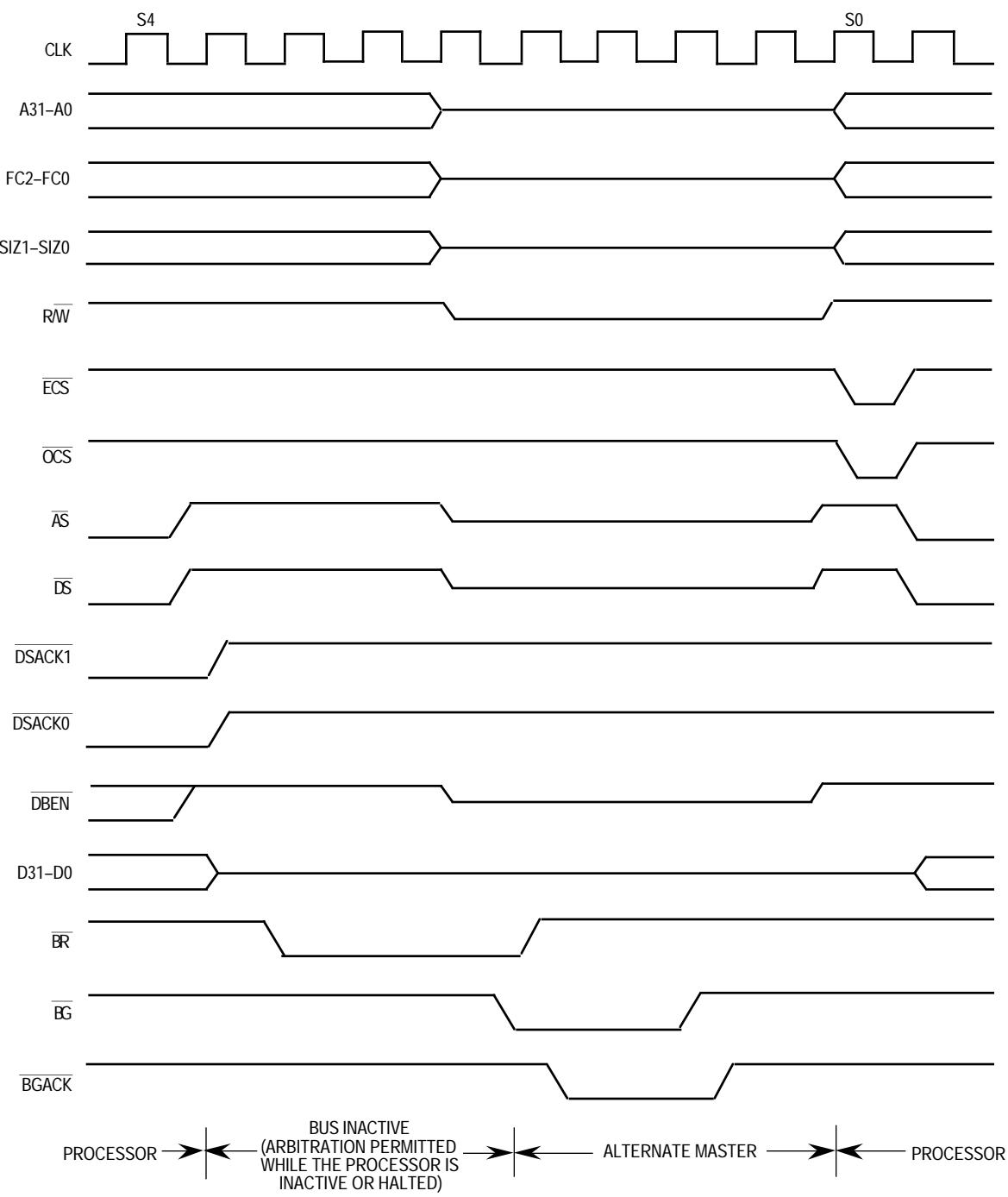
**Figure 5-45. MC68020 Bus Arbitration Operation Timing—Bus Inactive**
