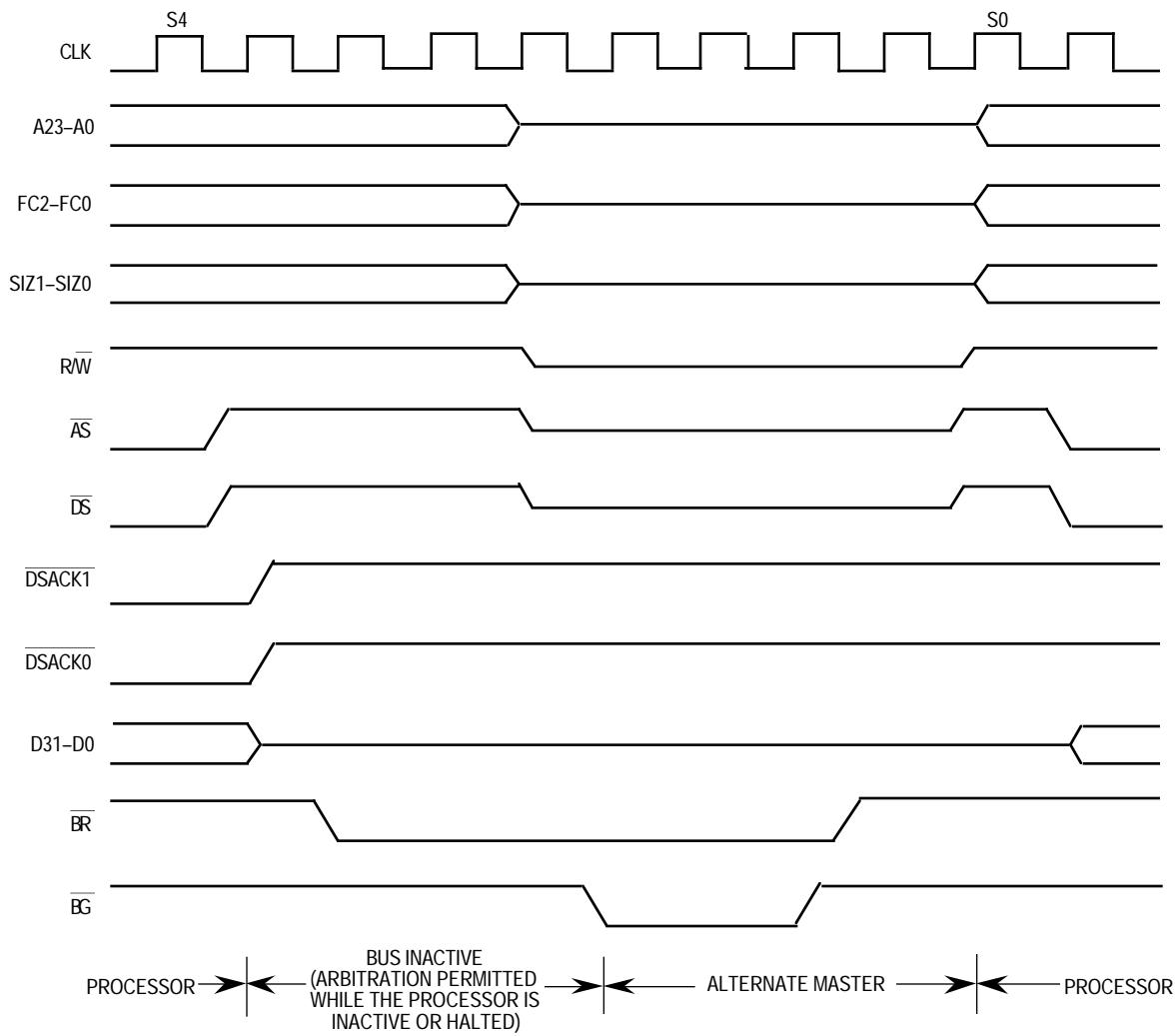
**Figure 5-49. MC68EC020 Bus Arbitration Operation Timing—Bus Inactive**
