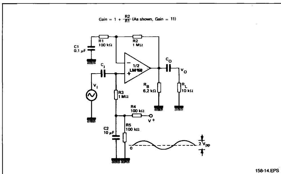
TYPICAL APPLICATIONS (single supply voltage)  $V_{CC} = +5V_{DC}$  (continued)
