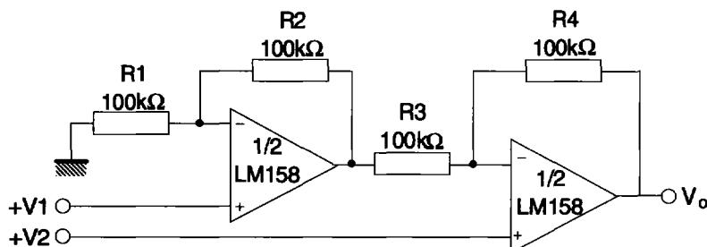
for  $\frac{R_1}{R_2} = \frac{R_4}{R_3}$  (CMRR depends on this resistor ratio match)
