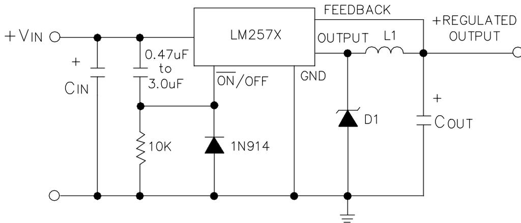
Circuit allows for  $C_{IN}$  to be fully charged before start-up, provides  $C_{IN}$  to supply hi-peak current instead of input supply.
