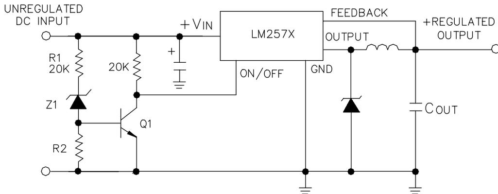
Regulator will be off until a  $V_{IN}$  set point is reached.
