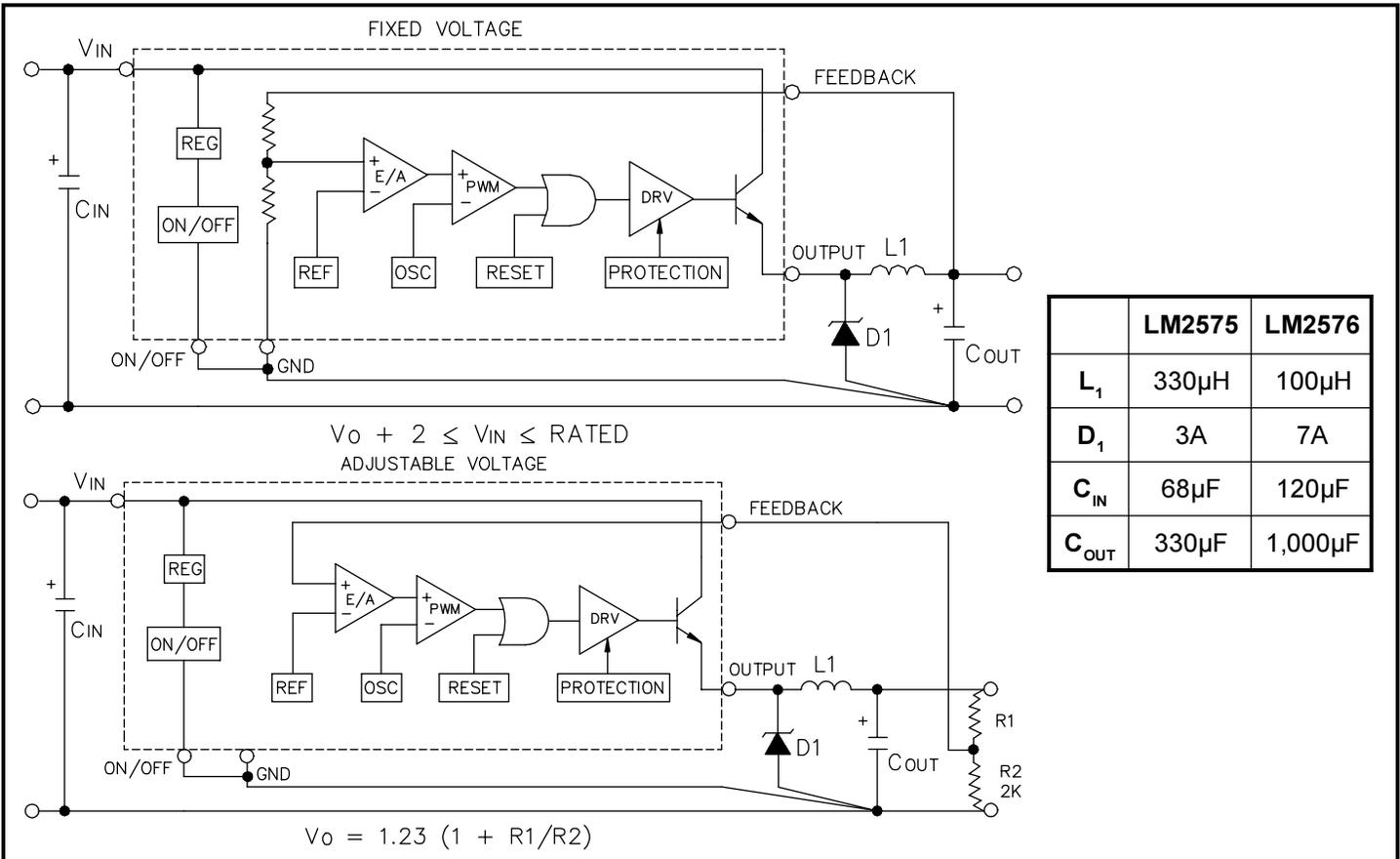
The above component selections will be adequate for most applications for output currents from 250mA to 3A (LM2576) or 150mA to 1A (LM2575). Applications with  $V_{OUT}$  below 5V or above 24V may require component adjustment for maximum performance; please contact factory for application assistance.
