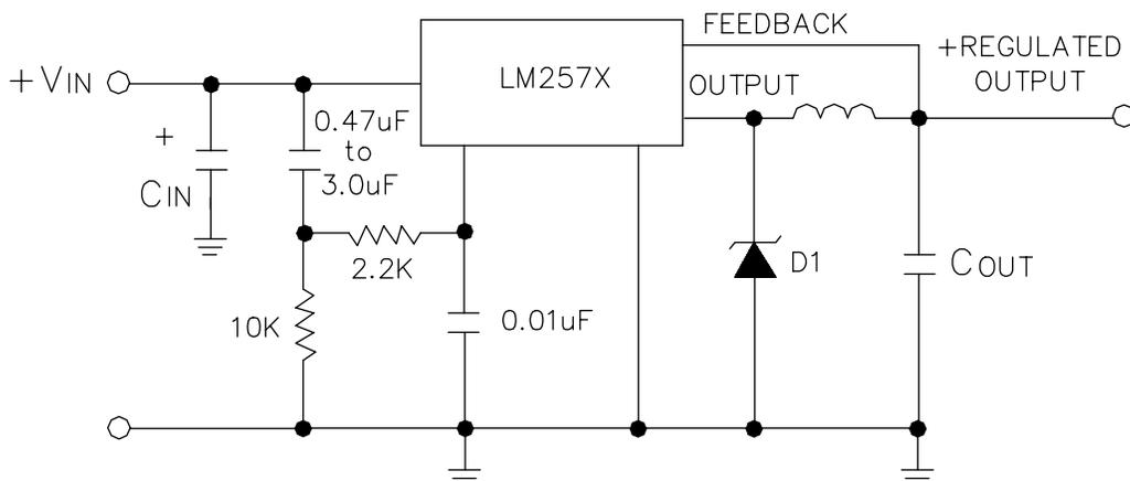
Spike filter reduces input noise, causing false triggering of delay.
