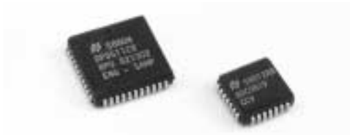
Molded Plastic Leaded Chip Carrier (PLCC)
