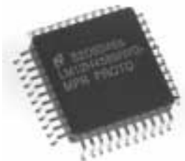
Ceramic Quad Flatpack (Gullwing) Product Suffix: WG
