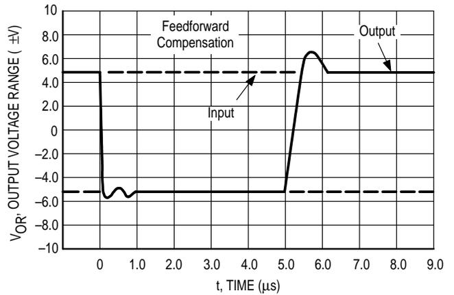
Figure 14. Single-Pole Compensation
