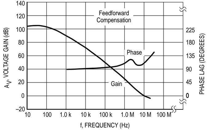
Figure 12. Large Signal Frequency Response
