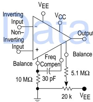
**Figure 2. Double-Ended Limit Detector**
