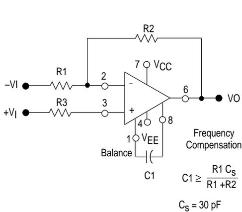
Figure 15. Feedforward Compensation
