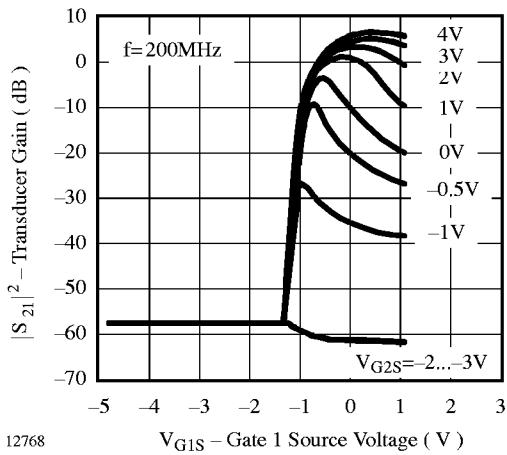
Figure 8. Transducer Gain vs. Gate 1 Source Voltage
