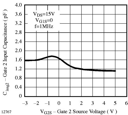
Figure 7. Gate 2 Input Capacitance vs.
