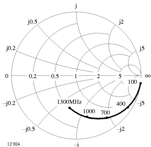
Figure 14. Input reflection coefficient
