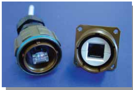
RJF TV Connectors for Ethernet Connection
