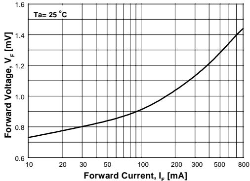
Figure 5. Forward Voltage vs Forward Current
