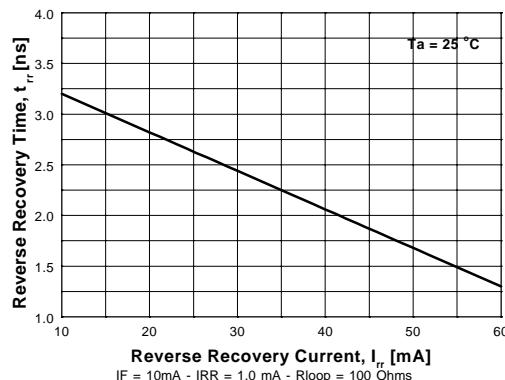
Figure 8. Reverse Recovery Time vs
