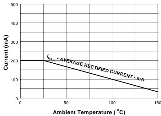
Figure 9. Average Rectified Current ( $I_{F(AV)}$ )
