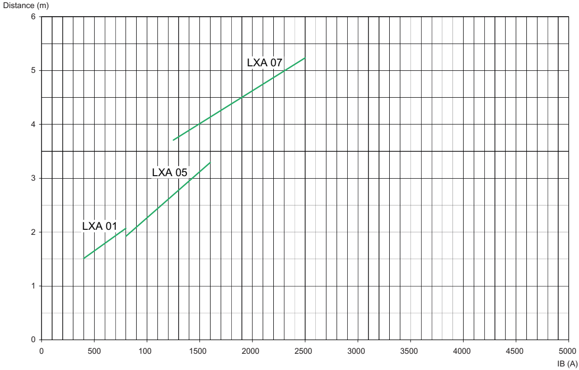
Figure 7-15 LXA load distance profile for 0.2 μT of systems 800 A, 1600 A and 2500 A
