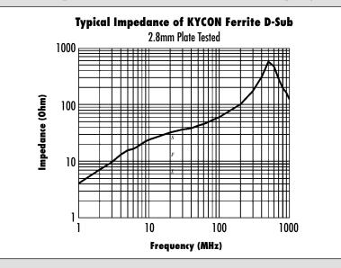
The above chart is typical performance data for a 2.8mm thick ferrite plate at room temperature. Impedance will be reduced by increased temperature (down approx. 15% at 100°C at 25MHz) and by increased DC bias (down approx. 15% at 1 amp at 25MHz). Also, impedance varies with ferrite thickness. Please contact our technical support for data specific to your application.
